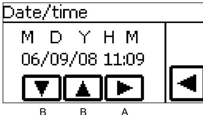
Button (A) can be used to make a selection and with buttons (B) adjustments can be made.
